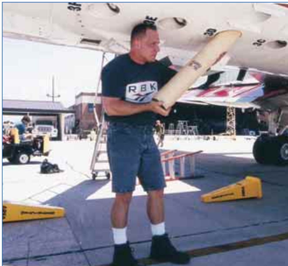
TECHNICIAN James Barr loads AXBTs into firing tubes. Explosives will shoot the probes clear of the plane during the flight.
